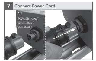
• Connect the whip end of the power cord to branch circuit. Align 3-pin female connector on power cord with 3-pin male input connector on luminaire and push into luminaire connector until firmly engaged.
