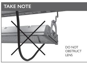
NOTE: Never position cords beneath the LED module(s), as they will obstruct the light output and light uniformity on the crop. Cords should instead, be positioned so that they can be secured to the mounting structure above the LED module, with a drip loop to draw moisture away from the connector.
