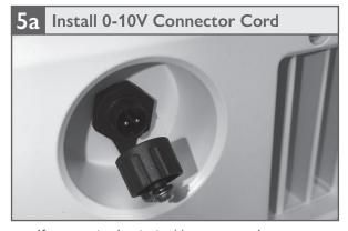
If connecting luminaire(s) to a control system, remove connector cap from 0-10V input connector on opposite end of luminaire.
