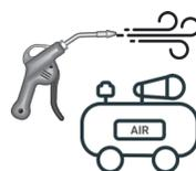
Use low pressure compressed air to remove dust and/or debris between the heat fins on the ballast housing.
