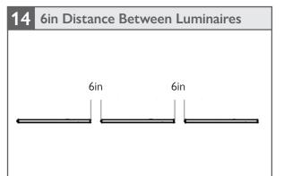
When luminaires are mounted consecutively, the distance between each luminaire must be a minimum of 6 inches
