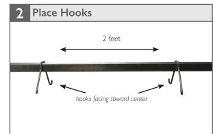
With hooks facing towards the centre of the luminaire, place both mounting brackets over the top of the track/truss in specified mounting location.
