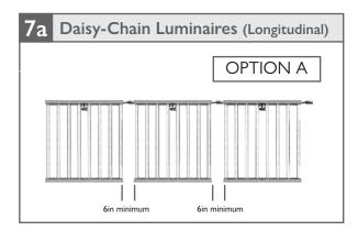
When luminaires are in a longitudinal orientation. the distance between each consecutive luminaire must be a minimum of 6 inches
