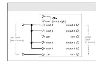
• Each signal board can accomdate up to four (4) inputs and four (4) outputs.
