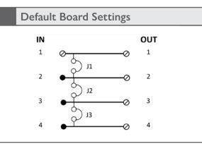
The default setting for each board is for singlechannel control, with all three (3) pre-installed jumpers in place—allowing for one (1) input signal to control all four (4) output signals.
