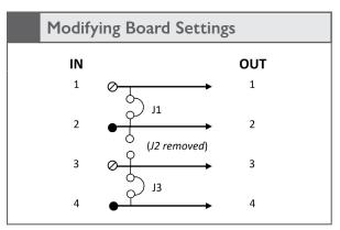
• To modify the number of channels used, simply remove the relevant jumpers on the board. For example, if two control-amplifying channels are required, then simply remove J2 from the board (see Modified Setting example above).
