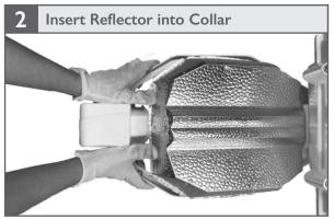
• Place open end of reflector over top of reflector bracket where it covers the lamp socket. Using thumbs, apply gentle pressure on closed end of reflector to lower and insert outer rim beneath the collar tabs. Note: Wear cotton gloves or wash hands thoroughly with soap & water to remove any grime/oils before handling reflector.
