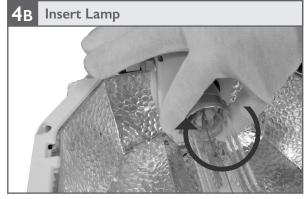
Holding the lamp by the metal ring at the base, insert into lamp socket and rotate clockwise until the lamp is securely installed
