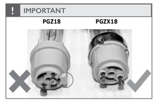
The NXT-LP CMH fixture is compatible with 315W open-rated / protected Ceramic Metal Halide (CMP) lamps ONLY. Compatible lamp types will be designated PGZX18.
